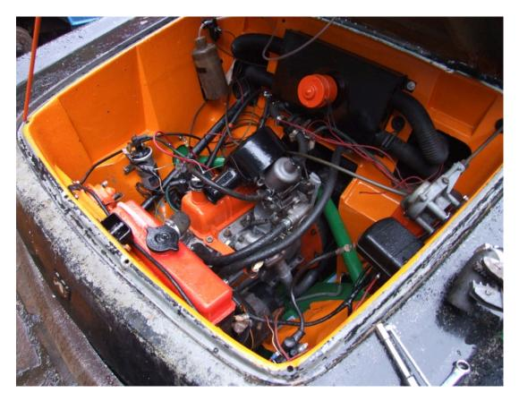
As you can see... at this point, there is no battery and it looks a bit untidy... The wiring seemed like it needed replacing, but instead, we cleaned all the bullet connectors and a few switches, and it came back to life... (you listening Colin? Ed)
