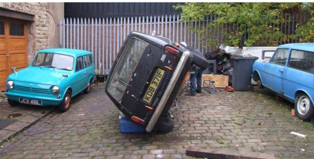
There is always the odd job that you wish you had done before the body goes back, but access is easy... a few empty 25litre plastic drums and then lift the car onto the oil drum pillows.
