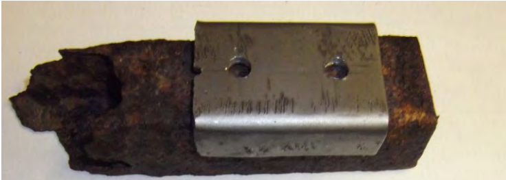
DRILLING JIGS MADE UP FOR DRILLING THE HOOPS IN THE BODYWORK
