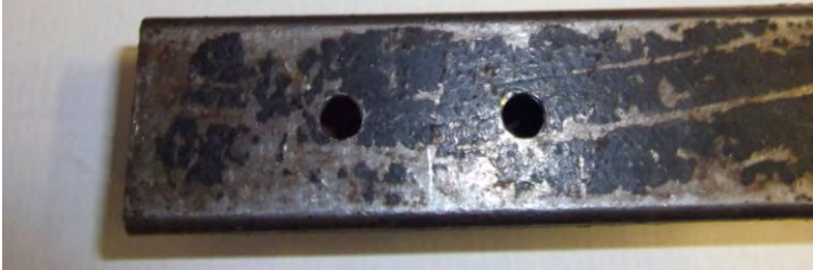
DRILLING JIGS MADE UP FOR DRILLING THE HOOPS IN THE BODYWORK
