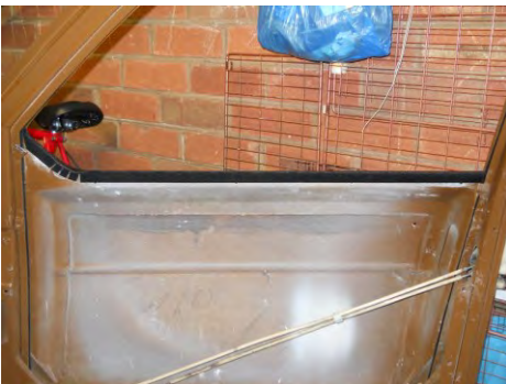
Pete's Kitten's drivers door during and after fitting of its new window sealing strip.
