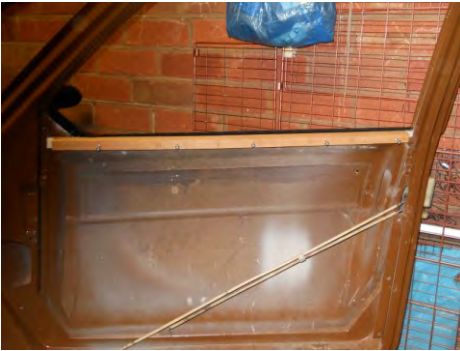
Pete's Kitten's drivers door during and after fitting of its new window sealing strip.
