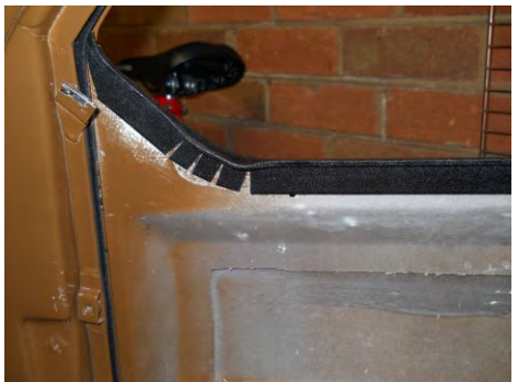
Pete's Kitten's drivers door during and after fitting of its new window sealing strip.
