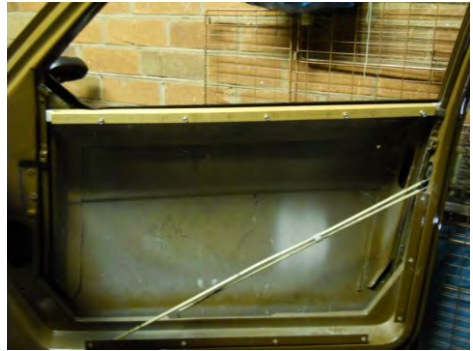
Pete's Kitten's drivers door during and after fitting of its new window sealing strip.
