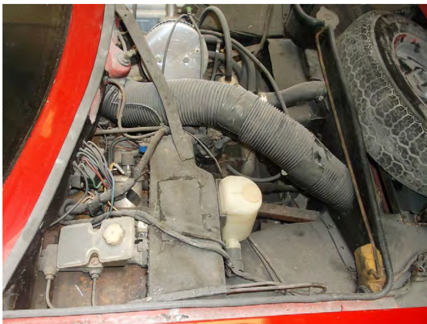
An under bonnet shot of No.1 – as it is completely original, I know many of us were taking notes! – the position of the fuse box is of great interest, since all later cars have it in the foot well – which is a bit harder to get too than No.1's fuse box.
