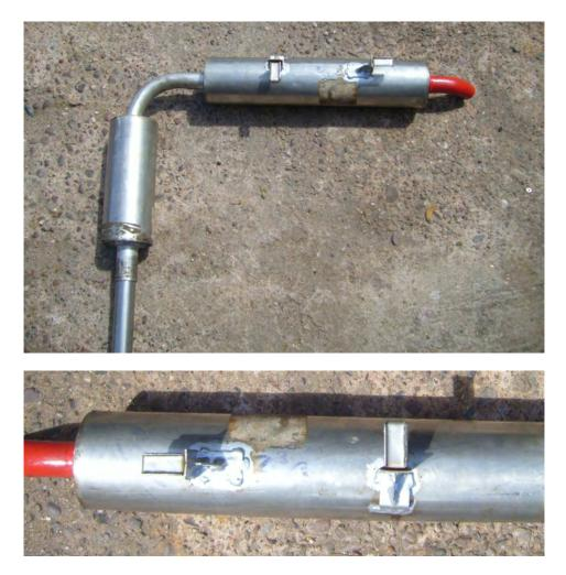
I just love the way those very capable engineering types use the language :- "using a 1500 MG Midget silencer box, 100 cm of 38mm diameter stainless tube, and you may need a pipe reducer to match pipe and manifold." He makes it sound oh so easy, which, if you have the skills and expertise I do not doubt it is, but for the rest of us mere mortals, well, it could present ever so slight a challenge I would imagine.
