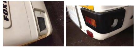
Now with the bumper paint dry, bolt the bumper back onto the Tandy. The rubber flap which was glued on before can now be rolled up to the inside of the bumper. Doing this will create a 'roof' over the socket on the inside of the bumper. Any water which comes down the body should now roll off either side of the socket. Before replacing the rear lights, I would recommend cleaning the connections, and applying some copper slip to them.
