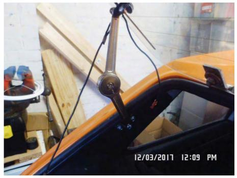
There's an Allen screw (on the far side in this picture) to adjust the amount of friction, and it was a doddle to set it to support the glass securely, with plenty of adjustment left should it loosen up in service, though it's been on there a couple of weeks now without problems. Also it looks good!!
