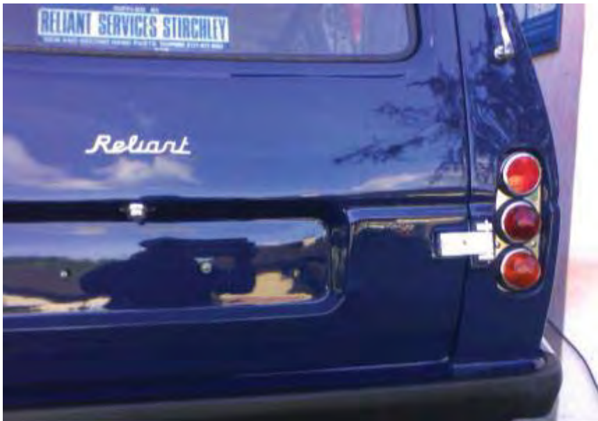
Just a few more pictures showing the gear lever and rear lights, the Reliant badge is made of water jet cut stainless, polished, and fixed with tiny m2.5 screws.
