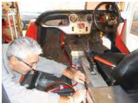
Alan runs the rather costly marine battery cable through the interior, it looks rather radical, and saves drilling lots of holes.
