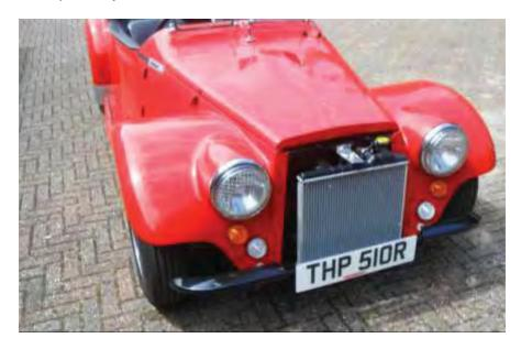
One piece of box section frame was removed making space for a pair of base brackets, fabricated with holes to accept the plastic positioning lugs. With the top secured by a similar steel plate, longer hoses were sourced along with fresh alloy tubing. Plumbed in, fresh coolant, plus a final oil change, and four months behind schedule she is done, and runs like a dream; its only taken three and a half years since I first found it languishing at the back of Professor Anthony Stevens unit in Kent.
