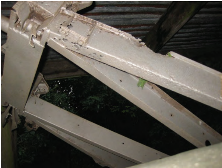
Chassis after blasting.
