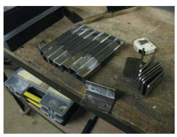
These gave a centre for the hole saw, and with a bit of care, and a slow speed on the drill, the tubes were drilled out.
