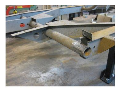
My solution was to turn up some discs with a hole in the centre, that were a good fit into the tube, and lightly weld them in place in the mouth of the tube.
