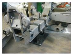
The chassis is now on the table and being bolted down. I have made a fixture to allow the very front cross member to be cut off and replaced in exactly the correct position. The cross member with the turrets is marginally better on my chassis than the one I got from Joe, so I'll repair mine in situ, and just replace the front one.
