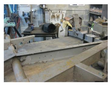
So, those were the plans, now for the action. If major sections of the chassis are to be removed, it is essential to put the chassis on a jig, and firmly bolt it down, so that no matter what happens, it cannot move.
