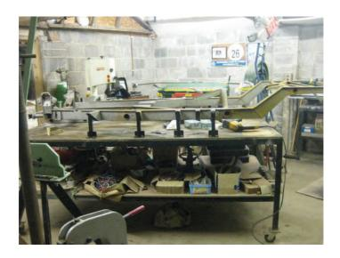
Cutting out could now commence. The side rail, "U" channel, and front cross member were removed. The very front cross member is mounted to the main one by inch and a half diameter round tube, and this needed to be replaced, which proved to be quite a challenge.
