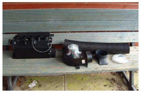
I did notice the foam on the direction flap had deteriorated, and that the water pipes where 5/8" diameter, rather than the usual  $\frac{1}{2}$ ". The motor was much larger, and it had a larger air pipe.
