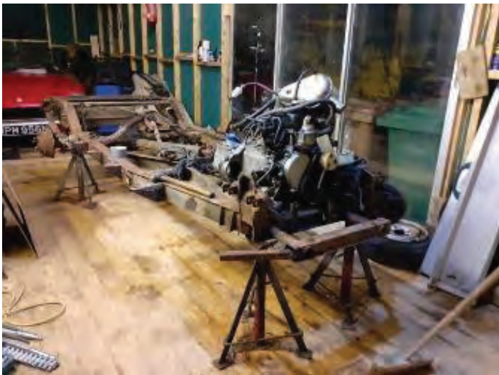
Here's the old chassis with the body and front suspension partly removed. Next, the new chassis, all painted up in primer ready for top coat.
