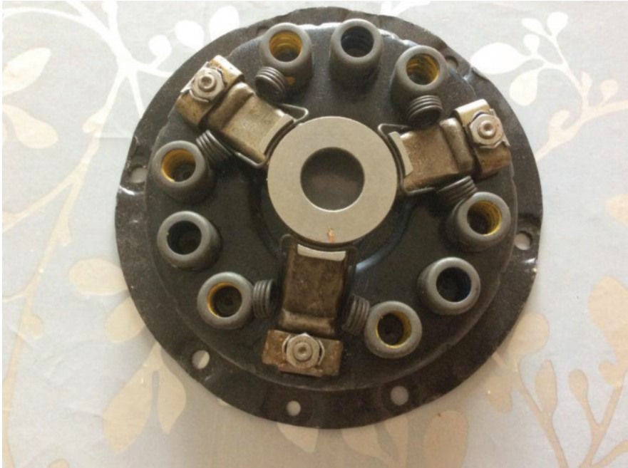
Phil's elusive 9 spring clutch cover assembly with 3 blue and 6 yellow springs
