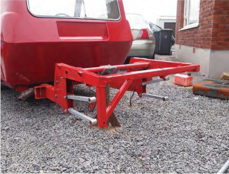
The body tub rear section has a box section that was an unused Rover P6 inner sill bonded in, this provides strength, and seat belt mounts. The cab is fairly roomy, with a rear seat (sort of crew cab?) this is across the back, and the extra fibre glass involved again braces the cab; the cushions were cut down from the original rear seat.
