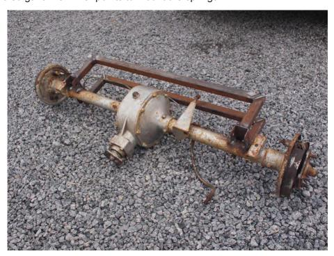
That decided, I had the propshaft lengthened and balanced, which gave me the extra 16 inches in wheelbase. The hand-brake system of rods was replaced with a metro cable, which uses a similar back plate, and was a fairly straightforward fit.
