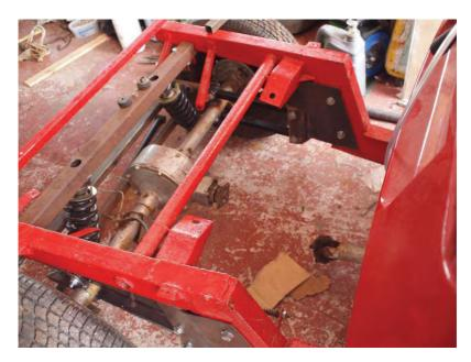
I had the chassis welded by a local professional fabricator, and there are tubes welded into the axle, to stop the suspension plates crushing it, or wearing holes oval.
