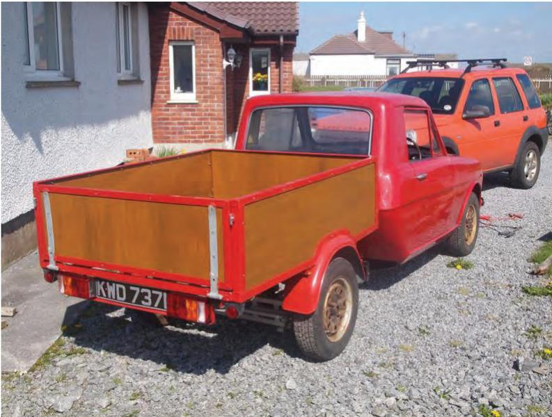
The back I welded up from 3mm angle iron, I let the trailer wheel arches into the back, so the that bed was not too high for loading, and the tail gate can be removed easily, when it is down for longer loads. There is a bit of an overhang, and loads of any significant weight need to be kept forward of the axle. The paint on the back is Hammerite red, with a little black added, to make it match the VW red of the body.
