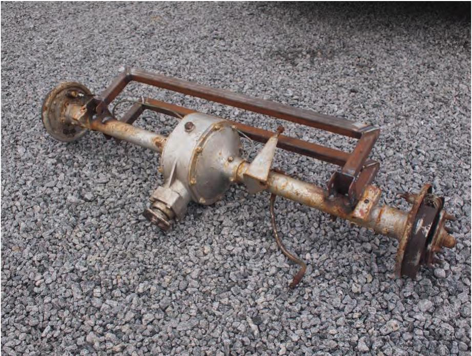
That decided, I had the propshaft lengthened and balanced, which gave me the extra 16 inches in wheelbase. The hand-brake system of rods was replaced with a metro cable, which uses a similar back plate, and was a fairly straightforward fit.
