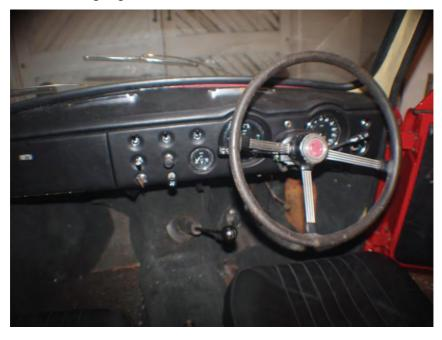
The additional switches for the interior light and parking lights came from my long-gone Rover P6. With a little heat, the vinyl is surprisingly easy to stretch. The windscreen demister vents were a bit rusty, and I managed to loose one, so I treated myself to reproduction MGA chrome vents, which fitted perfectly (Smiths heaters are a bit - one size fits all). I fitted a wiper motor from an MGB, which just required changing the drive cog to produce the correct sweep, then I was able to
