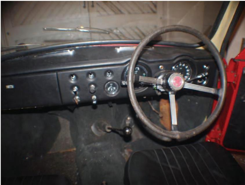
The additional switches for the interior light and parking lights came from my long-gone Rover P6. With a little heat, the vinyl is surprisingly easy to stretch. The windscreen demister vents were a bit rusty, and I managed to loose one, so I treated myself to reproduction MGA chrome vents, which fitted perfectly (Smiths heaters are a bit - one size fits all). I fitted a wiper motor from an MGB, which just required changing the drive cog to produce the correct sweep, then I was able to
