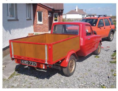
The back I welded up from 3mm ankle iron, I let the trailer wheel arches into the back, so the that bed was not too high for loading, and the tail gate can be removed easily, when it is down for longer loads. There is a bit of an overhang, and loads of any significant weight need to be kept forward of the axle. The paint on the back is Hammerite red, with a little black added, to make it match the VW red of the body.
