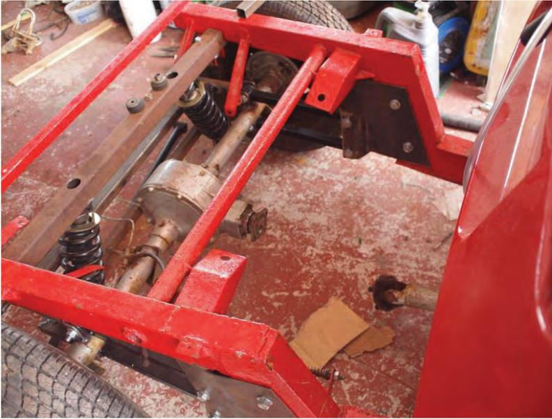
I had the chassis welded by a local professional fabricator, and there are tubes welded into the axle, to stop the suspension plates crushing it, or wearing holes oval.
