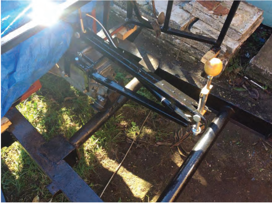
Before and after the remote gearchange mod and bulkhead painting.
