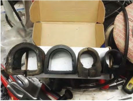
The old rack bushes beside the new Poly ones.
