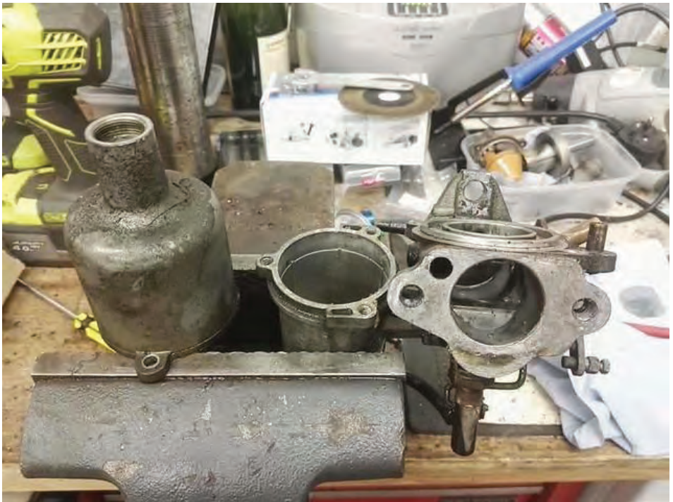
The carburettor was stripped, cleaned, and rebuilt, with a kit from the SU specialists, Burlen Fuel Systems of Sailsbury.
