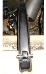
Testing again after showed the hinge to latch together in vertical position and to drop freely to the locking position. Pin width was then cut off either side to match the hinge profile and cleaned up with a file.
