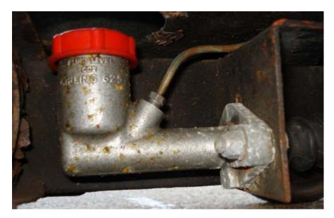
Thanks for the pictures. I see that the body bears the markings "CC2" and "G25". I think that G25 is the casting type and any replacement Girling master cylinder of the correct size should carry this reference. Be aware that the bore size could be different though, because there was nothing to stop Girling from boring out the same standard casting with different bore sizes.
