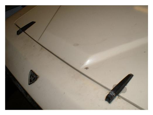
Final result. Note existing damage around hinge area caused by flapping about over last 24 yrs. Now the hinge is secure in closed position and bonnet lock is still effective. Hinges cannot lift because slots are cut down in each hinge.
