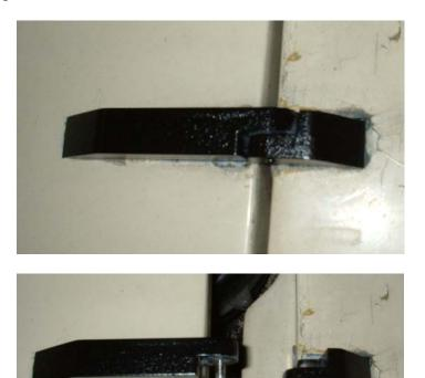
As can be seen they consist of "half hinges" with pivot pin and are now of solid bar construction instead of cast construction. I still prefer to be able to "whip off" the bonnet when required, for easy access to engine bay.
