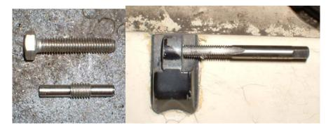
The hinge section was then tapped M6, no drilling is required this can be done in position, make sure you keep the tap square using a small adjustable spanner to turn.
