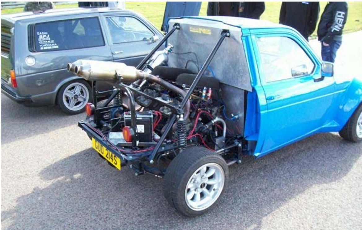
David Firman's blue converted van used a Suzuki V twin 1000cc engine, but then he discovered that some other Kittens were faster, so he moved it over and back a bit, and fitted a second one!
