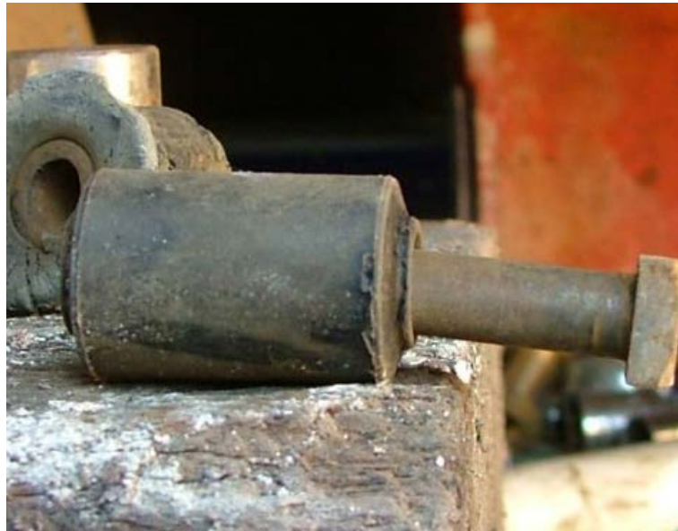
You can also see how slack the bolt is in the "normal" bush.
