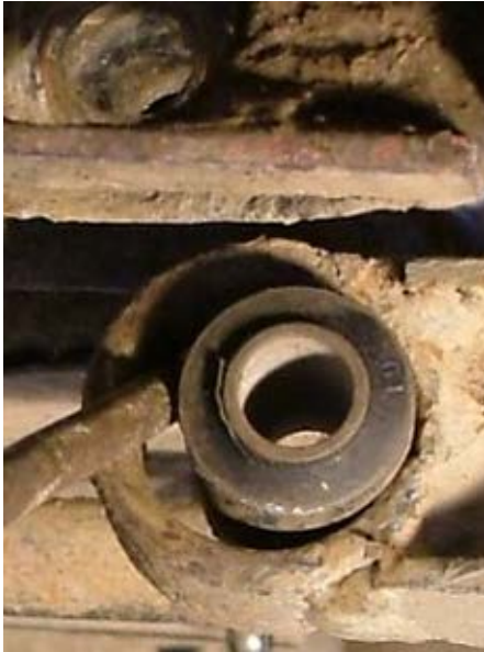
You can see above just how slack the 'normal' bush is!
