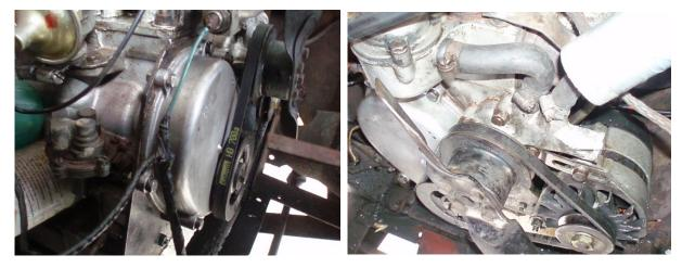
Observant enthusiasts will spot the redundant mechanical fuel pump, must remember to get a blanking plate and remove the old pump, I often wonder how much energy is wasted cranking its operating lever up and
