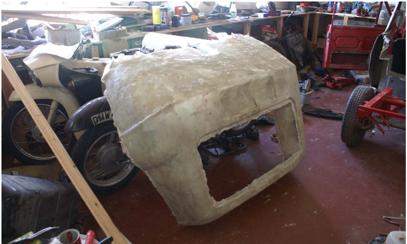
The mould for the new cab rear, (above) and the resulting panel (over)
